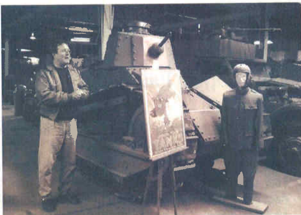
Joe McClain discusses his museum's oldest tank, a World War I vintage U.S. copy of a French Renault design. It carries two men and offers a top speed of only 3.4 mph.
