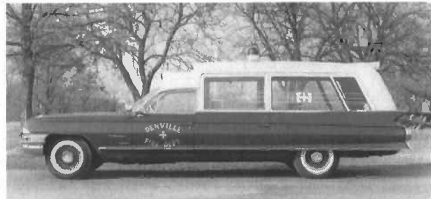
A "two-step" roof with oval S&M tunnel lights was employed for this truly-unique 1961 Cadillac constructed for Denville, N.J.'s F.D. by National Coaches of Knightstown, Indiana. Profound thanks to Roger White, M.D. of Rochester, MN for sharing these rare images.
