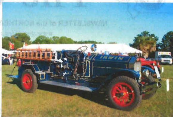
Vintage fire trucks in the "Quest for Speed and Style" exhibit at the 2007 Hilton Head Concours included this company-owned 1928 American LaFrance 1,000 G.P.M. pumper originally used in Irwin, PA.
