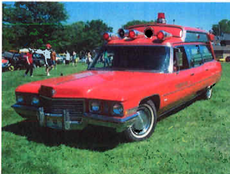
An interesting Lahaska newcomer was the Washington, N.J. Emergency Squad's 1972 S&S Cadillac Medic Mark I ambulance, which employed "West Coast" mirrors and externally-mounted quarter window nameplates.
