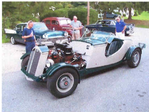
Finished one month prior to the PCS Mid-Atlantic Chapter's visit to his shop, Ross Miller's "Speedwell Roadster # 1" required three years of work to finish in his spare time, as well as whole lot of repurposed Packard parts. The engine is a 1951 "Thunderbolt" inline eight displacing 288 cubic inches.
