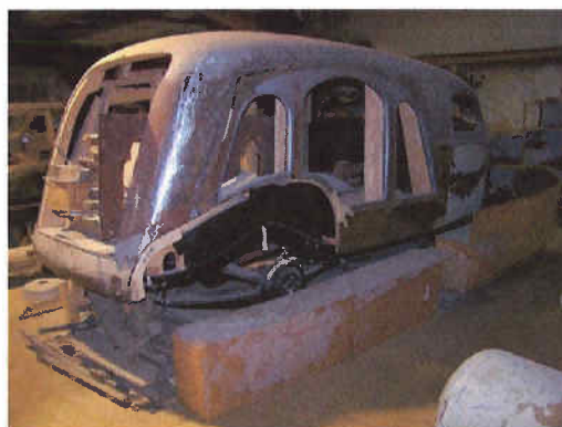
This 1937 S&S Buick Byzantine carved panel hearse, owned by Wilkes-Barre, PA funeral director and CRITERION Publisher Ted Collins, was in this state of disassembly when the Mid-Atlantic PCS visited Penn-Dutch Restorations in August, 2010. Though the restoration entailed replacing most of the ash wood framework due to termite damage, it's supposed to be finished in time for the 2011 International Meet taking place in Hudson, Ohio this July 12th through 16th.
