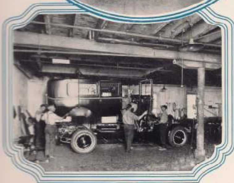
In view on the left is a completed body being lowered onto the finished chassis—and made ready for final test and inspection.
